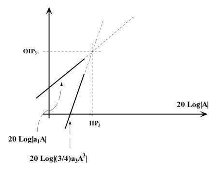
IP3 is the "third order intercept point". IIP3 is "input IP3" and OIP3 is the "output IP3". IIP3 is the value of the input amplitude where
