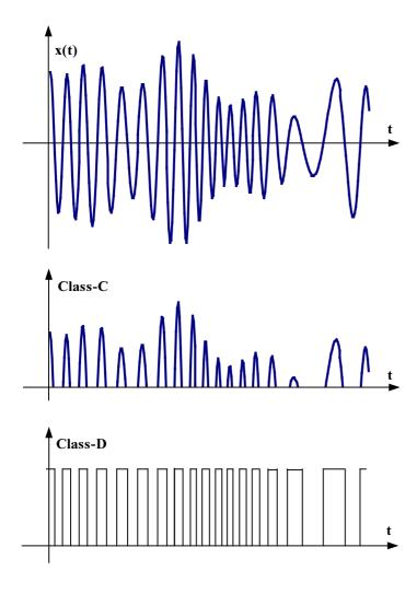
The nonlinearity in Class-C and Class-D amplifiers are severe. Coefficients  $|a_2|$  and  $|a_3|$  can be as large as  $|a_1|$ , sometimes larger than  $|a_1|$ . The relevant part of output becomes
